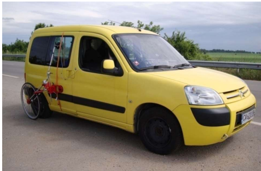
Figure 5. The converted vehicle, equipped with "fifth" wheel during the tests
