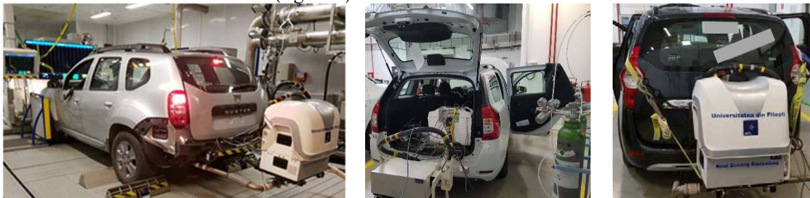
Figure 3. PEMS mounting on vehicles
