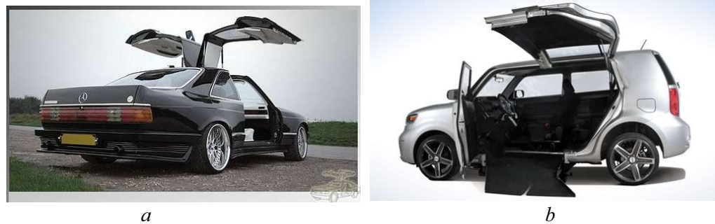
Figure 4. Doors [12] with horizontal axis, type gull wings : “coupe” (a) and at rear (b)
