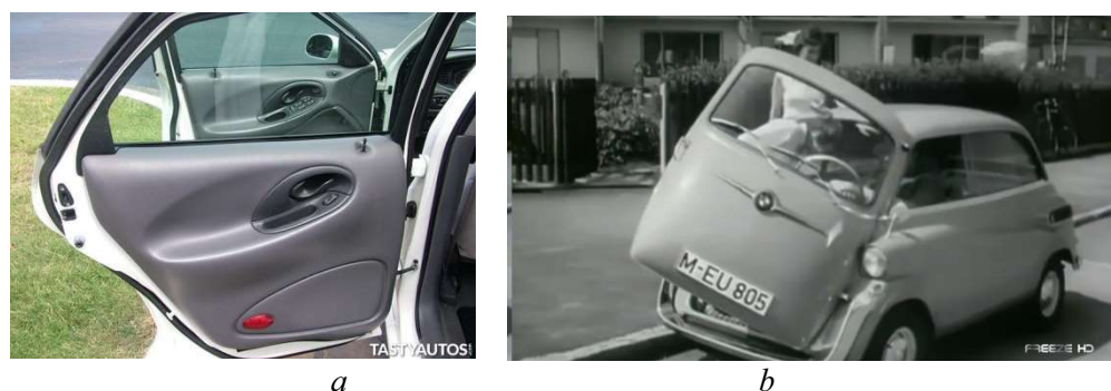
Figure 3. Conventional vehicle rotate doors [11, 12] with vertical axis hinges (a) and front vehicle rotate door with inclined axis hinges (b)
