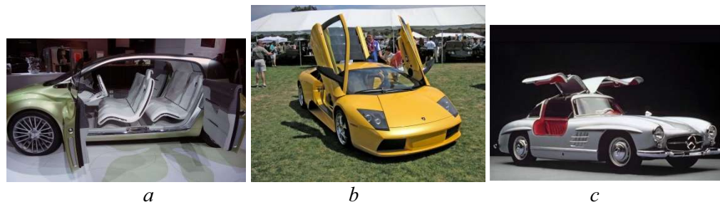
Figure 1. Unconventional car doors ( a – suicide, b – scissors, c – gull wings) [11, 12]
