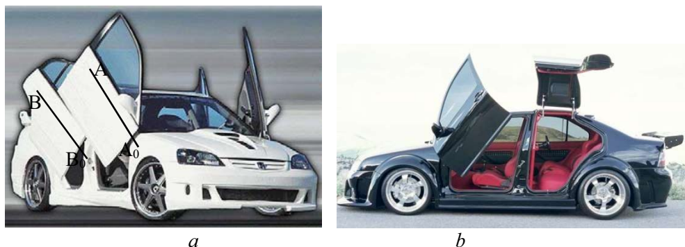
Figure 7. Photos [12] with rotate doors in a longitudinal-vertical plane, type scissors : front/rear (a) and only in front (b)
