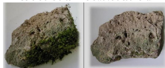
Figure 3. Yellow tuff sample attacked by musk before and after microwave treatment.
