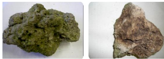
Figure 1. Grey tuff sample attacked by lichens before and after microwave treatment.
