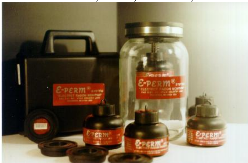
Figure 5. E-Perm® system for Radon activity concentration measurements[7].
