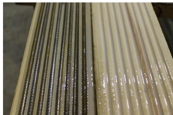
Figure 6. Reinforcement gluing-in process.
