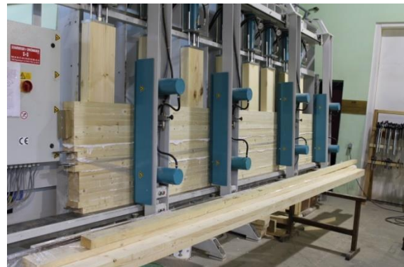
Figure 8. Specimen pressing and curing.
