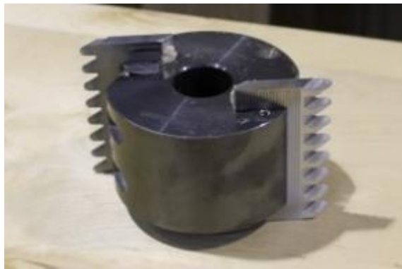
Figure 7. The milling cutter for groove milling.
