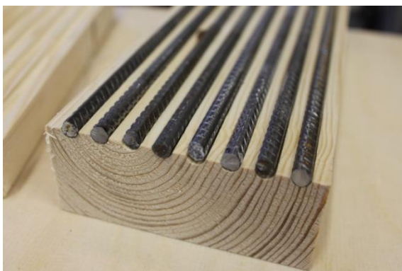
Figure 5. Specimen with double-faced groove.
