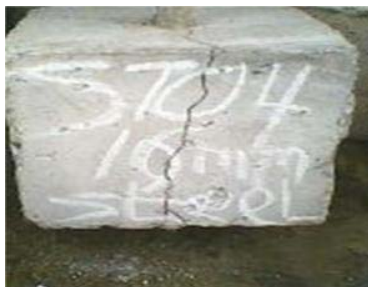
Figure 2. RILEM specimen that failed by splitting.
