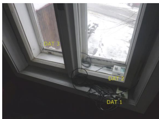
Figure 3. Placement of dataloggers and probes on the double casement window.
