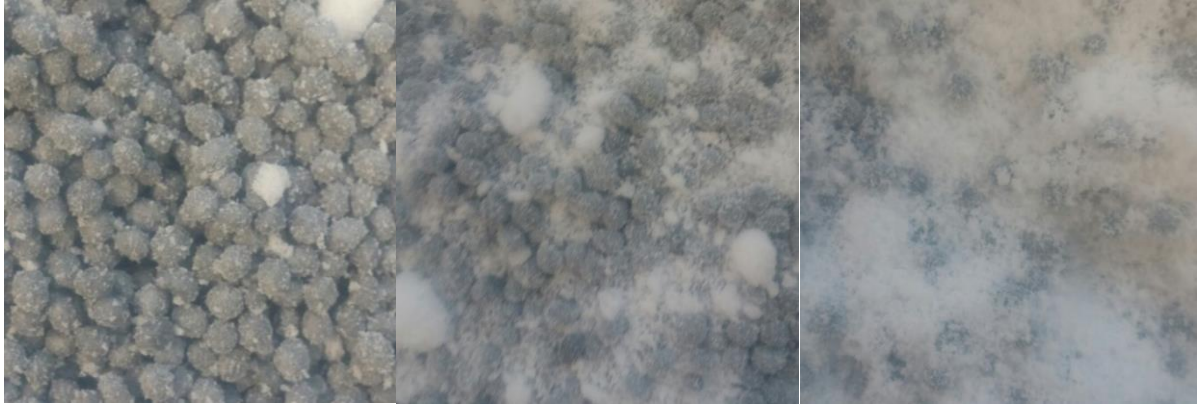
Figure 1. Photographs of Izoprol and Izoprol material mixtures. Left – \eta=0.12 , middle - \eta=0.46 , right - \eta=0.73 .
