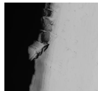
Figure 5. AFM Tapping Phase image of untreated hemp fiber 40x 40µm [11].
