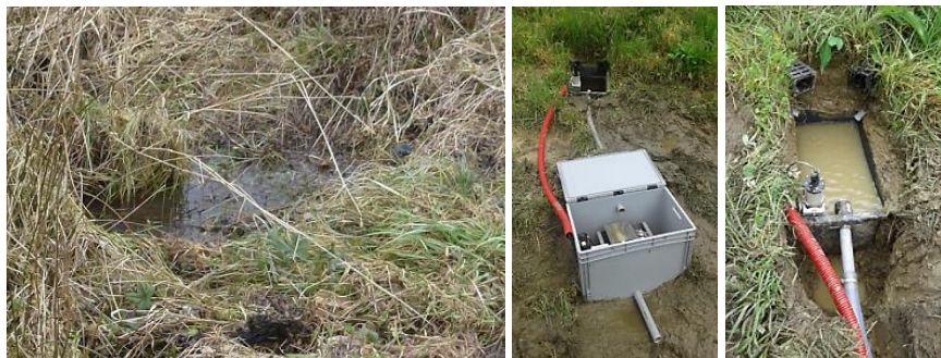
Figure 5. Detailed view of the place of seepage with the clear water inrush and the system measuring seepage, temperature, electrical conductance and pH of seepage water.
