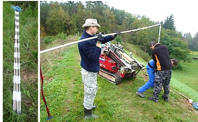
Figure 3. Detailed view of the EIS3 probe, installation of the EIS10 probe using a Pagani rig.
