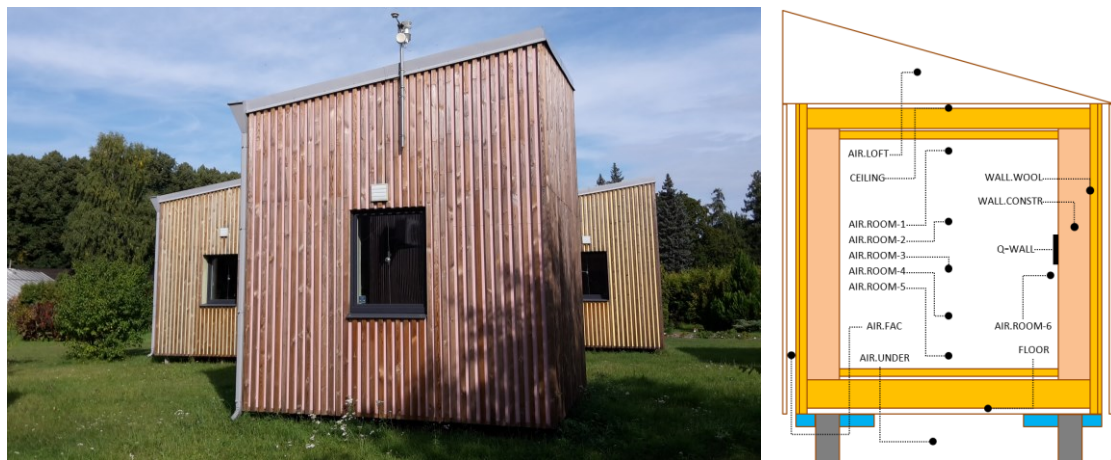
Figure 1. Overview of the testing ground and cross-section of the building with the location of main temperature and air humidity sensors (marked as dots) and heat flux sensor (Q-WALL).
