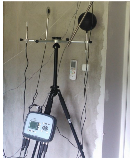
Figure 4. Microclimate measuring device DeltaOHM HD 32.1 with radiant temperature asymmetry and globe temperature sensors.
