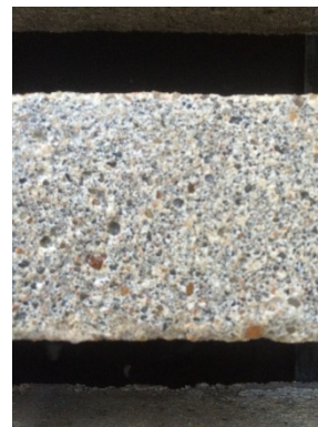
(D) Mortar appearance protected by corrosion resistance admixture CY
