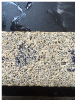
(C) Mortar appearance protected by aluminate cement KS
