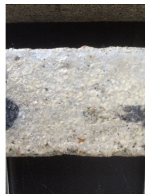
(B) Mortar appearance protected by NF sealer
