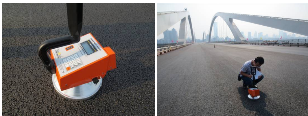
Figure 7. Using Pave Track TM Plus to Collect the Data of Compactness
