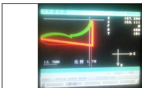
Figure 6. The cutting tool route on the numerical control panel.
