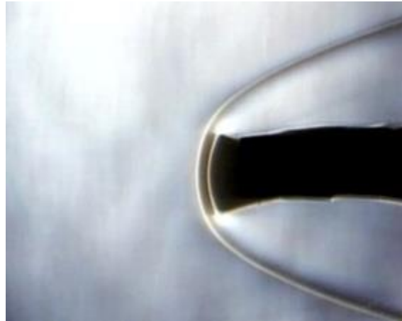
Fig. 5. Schlieren image of the flow field with no jet injection
