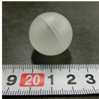
Fig. 3. Photograph of projectile, which diameter is 25.75 mm, mass is 4.3 g, respectively.
