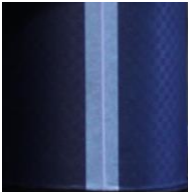
Figure 6. A thread with adhesive tape simulating a stitch
