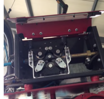
Figure 9. The welding machine of PHOENIX 522. Figure 10. The wire feeding mechanism.
