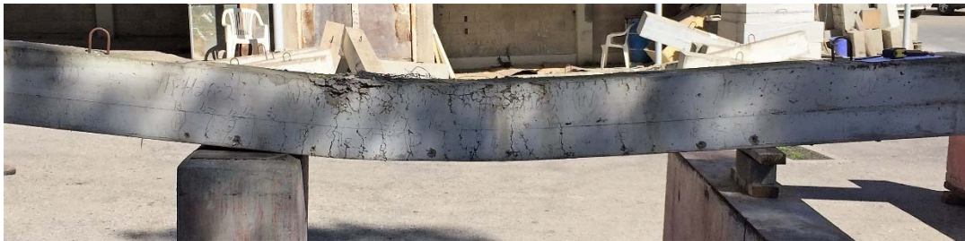
(b) No cracking localization in specimen NF-1-126 ( \rho = 1.26\% )
