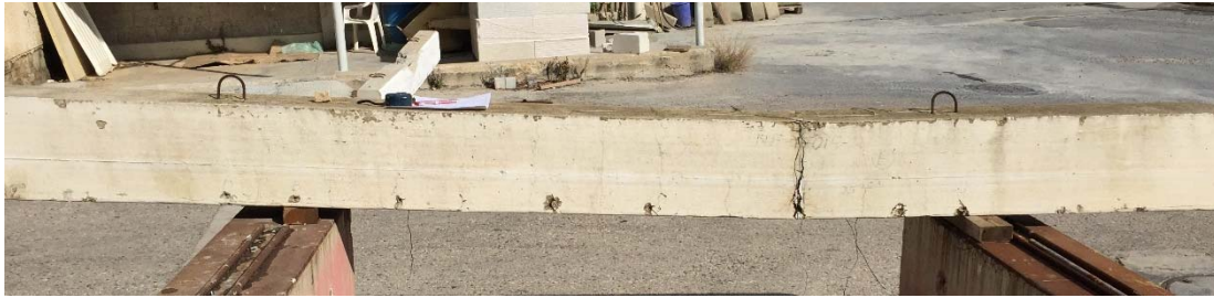
(a) Cracking localization (single wide crack) in specimen NF-1-015 ( \rho = 0.15\% )
