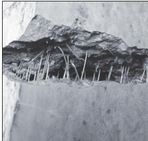
Figure 1. Tension fracture of a beam with pulled out fibers
