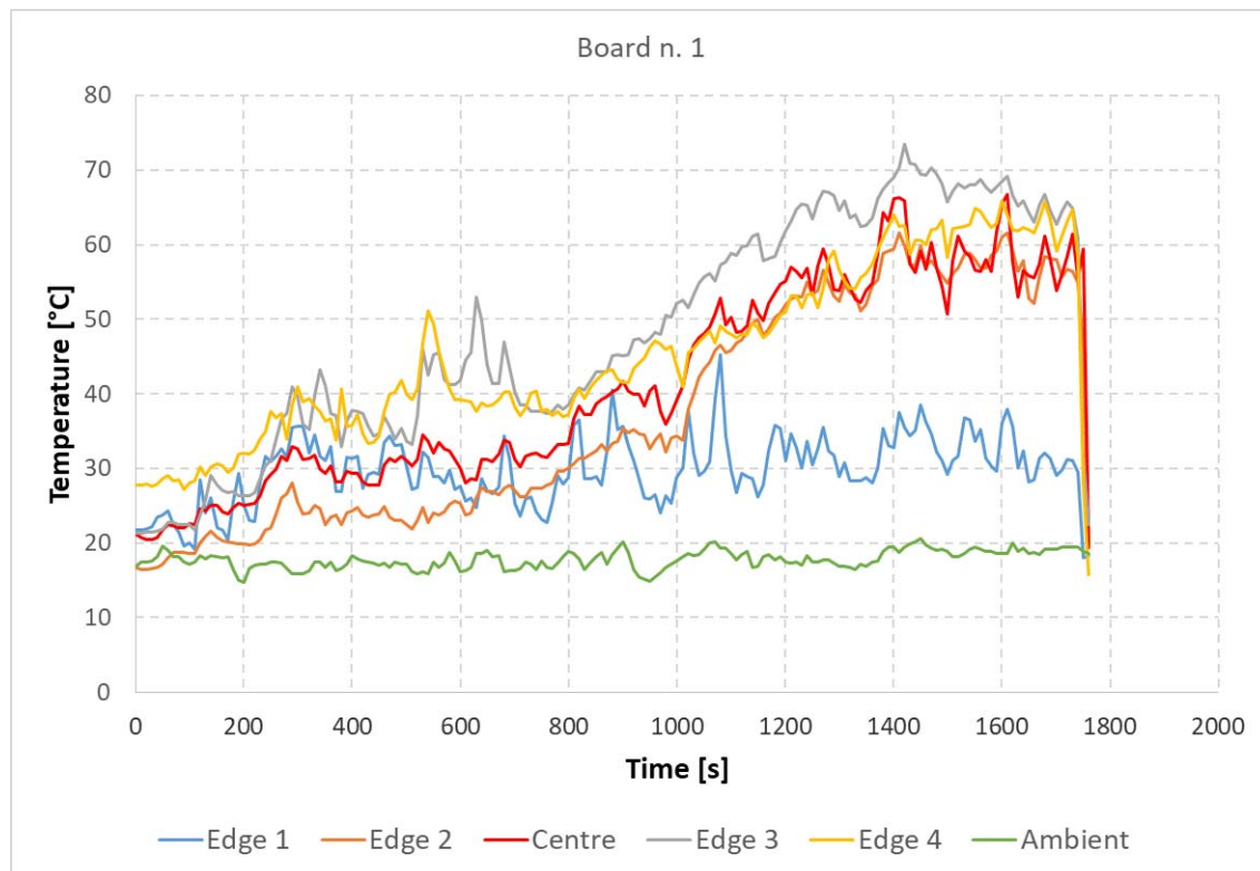
Figure 5. Results of temperature measuring in the test of board 1.
