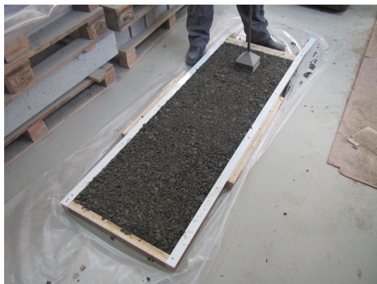
Figure 3. Compacting of the board by compactor.
