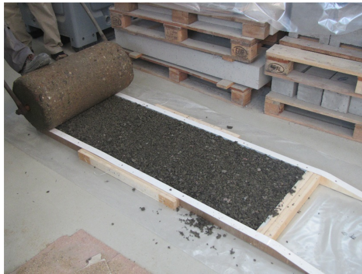
Figure 2. Compacting of the board by rolling.
