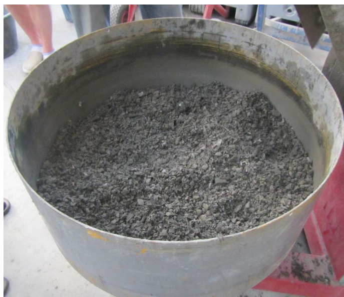
Figure 1. Fresh concrete composite with textile shred.
