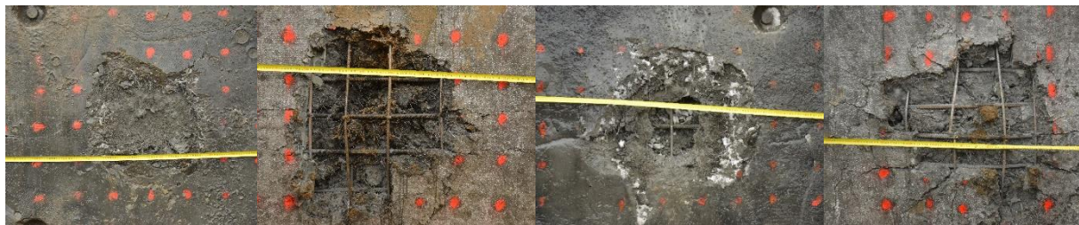
Figure 12. Specimen No. 23 after contact blast loading, 2.8 kg charge left left contact side, left right soffit, 4.2 kg charge right left contact side, right right soffit
