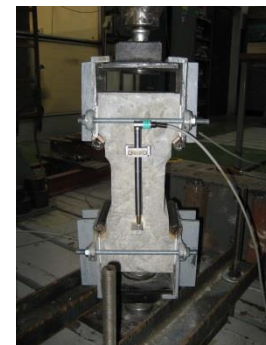
Figure 6. Axial tension test - dogbone
