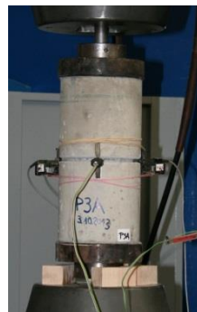
Figure 5. Axial tension test - notched cylinder
