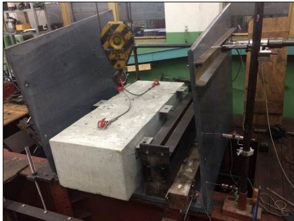
Figure 6. Test of load bearing capacity of the right thin wall – an inward direction
