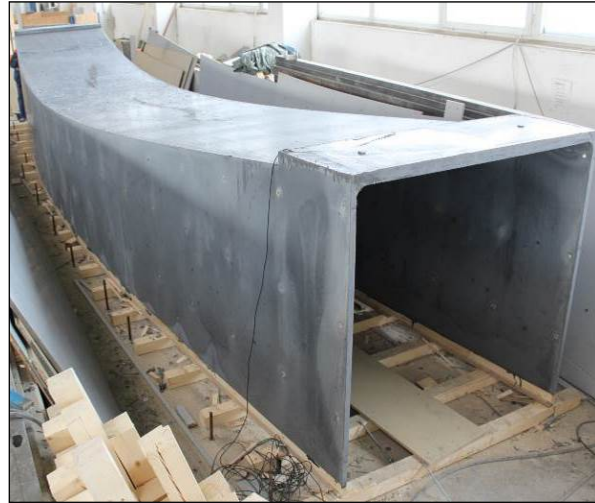
Figure 11. Final footbridge after demoulding
