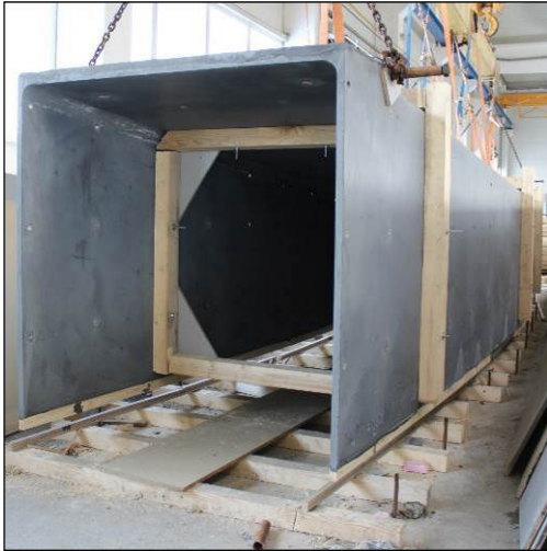
Figure 10. Demoulding of footbridge
