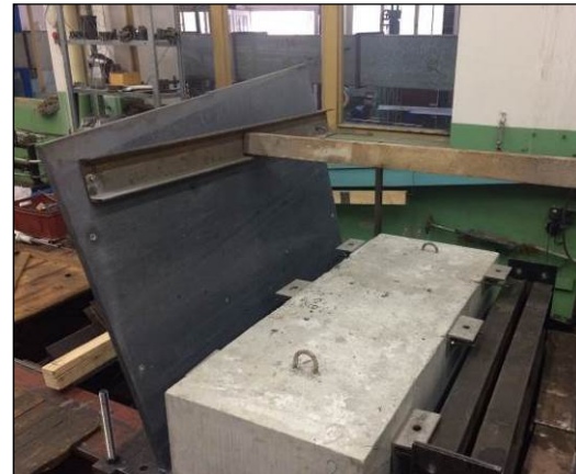
Figure 7. Test of load bearing capacity of the left thin wall – a way out direction
