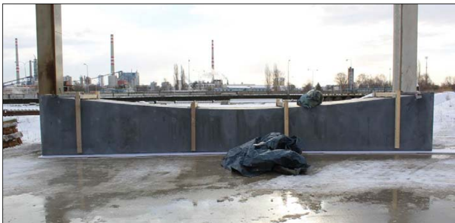
Figure 13. Storing of final 1:1 mock-up of the footbridge in upside-down position
