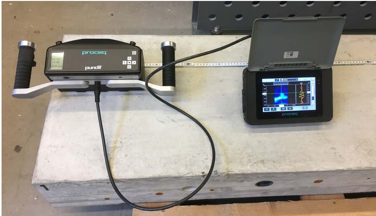
Figure 8. Pundit 250 Array Ultrasonic Pulse Echo Instrument
