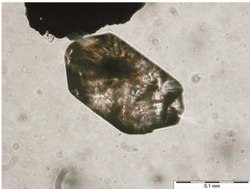
Figure 5. Zirconium mineral found in the studied rocks. Polarizing microscope 1P.
