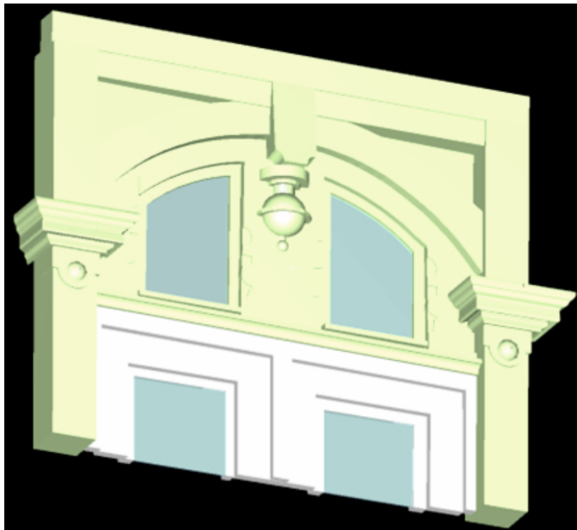
Figure 7. Models of architectural features created using the surface matching method on a point cloud measured at the highest resolution
