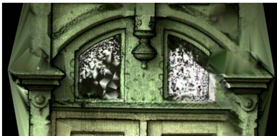
Figure 8. A model of a feature created using the TIN method on a point cloud measured at the highest resolution
