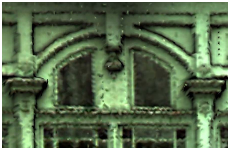
Figure 6. A model of a fragment of the veranda created based on the TIN method - the point cloud measured at a medium resolution
