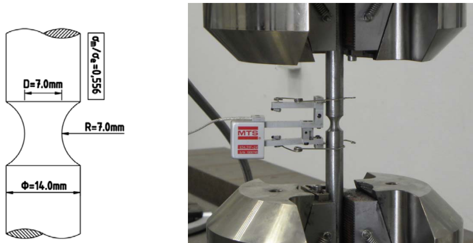
Figure 2. Geometry of cylindrical tensile specimens with a circumferential notch and view of the tensile test in multi-axial stress case
