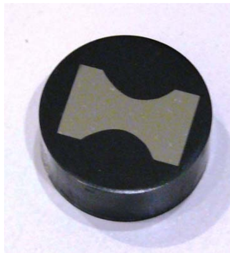
Figure 5. Metallographic specimen used in microscopic investigations
