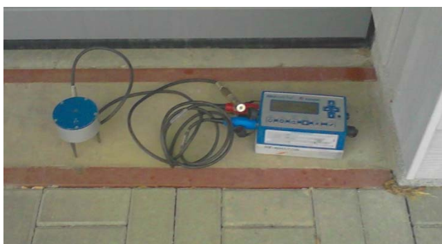
Figure 1. Monitoring of vibrations
