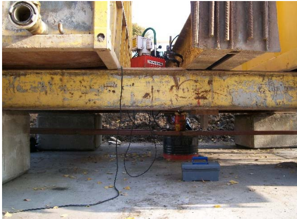
Figure 5. Static load testing
