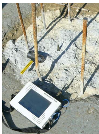
Figure 3. Testing of integrity by means of PIT method
