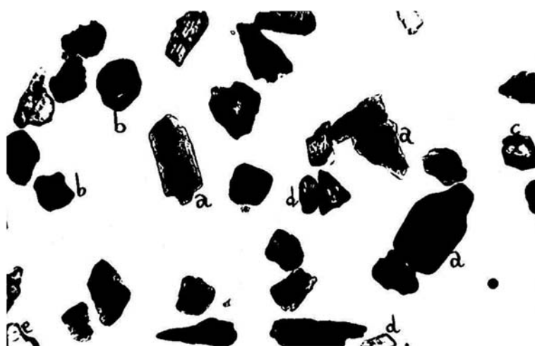
Figure 3. Assembly of heavy mineral from the sandy fraction of soil from Visag –350cm depth, cls.0,10-0,05mm; X70 parallel nicoli
