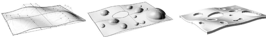
Figure 10. Modelling the free-surface with the Rhinoceros software
