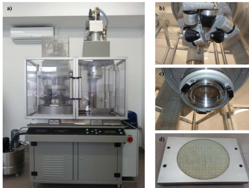
Figure 1. a) The FAP test equipment b) polishing rotary head, c) friction measuring rotary head, d) glass control plate
