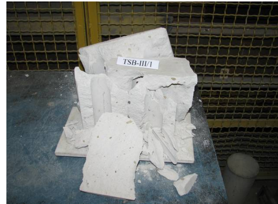
Fig. 5 Relationship of tested masonry units from TSB-I and TSB-III series: a) \sigma_{rad,I} = \sigma_{rad,II} = \text{const.} , b) \sigma_{ver} = \sigma_{rad,I}
