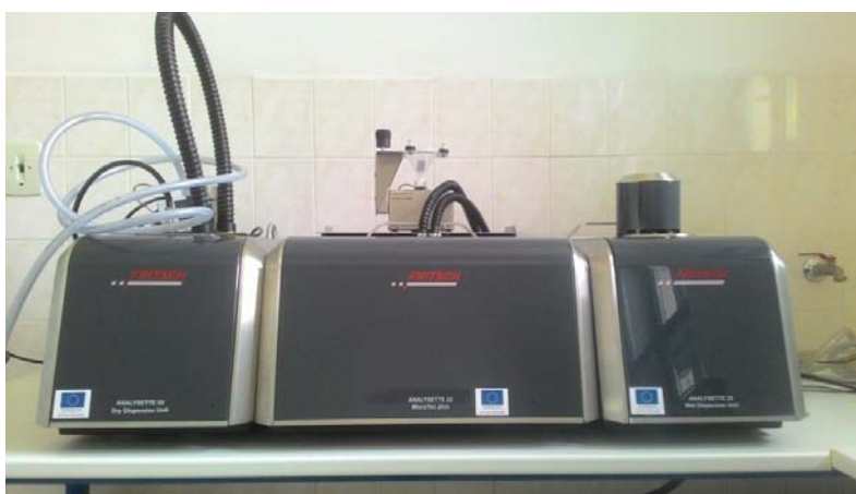
Figure 3. Laser analyzer ANALYSETTE 22 MicroTec plus (left to right): unit for dry samples, measurement unit and the unit for wet samples
