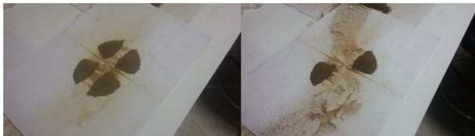
Figure 2. Procedure of quartering method
