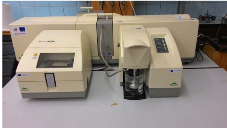
Figure 5. Laser analyzer Mastersizer 2000 (left to right): dry samples dispersion unit (Scirocco 2000), optical bench and the wet samples dispersion unit (Hydro 2000 MU)
