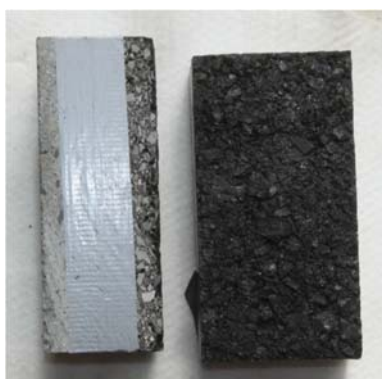
Figure 3. Test Specimen with Side Sealed Edge. Source: Author's compilation
