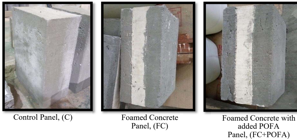
Figure 1: Assembly of three full-scaled panels
