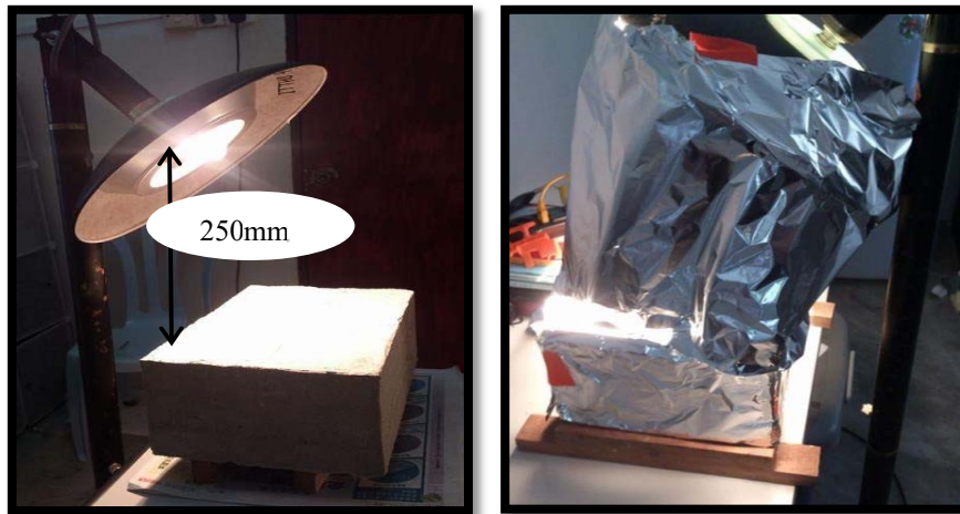
Figure 2: A schematic diagram showing the specimen, heat source and experimental setup before and after covered with aluminium foil
