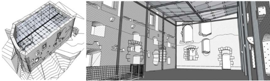
Figure 3a. Steel support structure with frames in cross-sectional direction with point fixed glazed tables allows to create open space.
