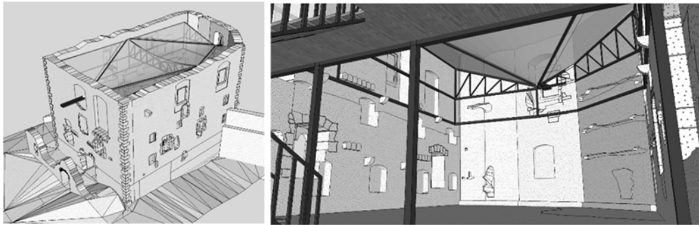
Figure 3d. Steel roof structure is laid on existing stone embedding in perimeter walls, the interior is free, roof covering is presumed as translucent textile membrane.
