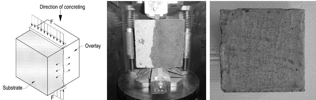
Figure 1. Model of specimen used in tests of tensile bond strength and substrate surface prepared with steel brush
