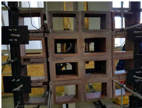
Figure 13. Failure of element of series I
