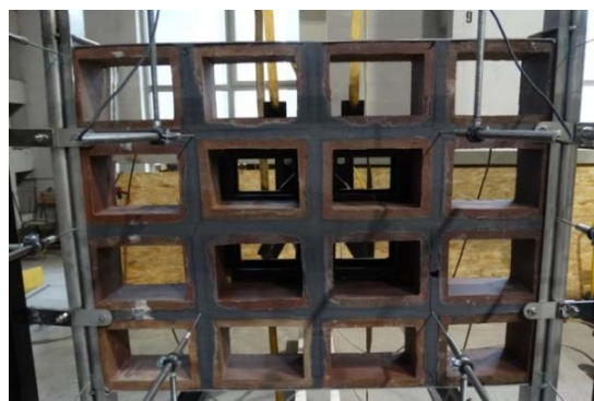
Figure 15. Pattern of cracks at maximum load
