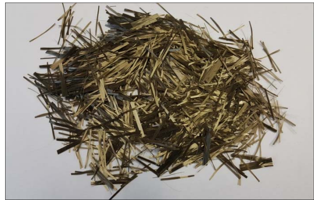
Figure 2. Polymer-basalt fibres (24 mm length)
