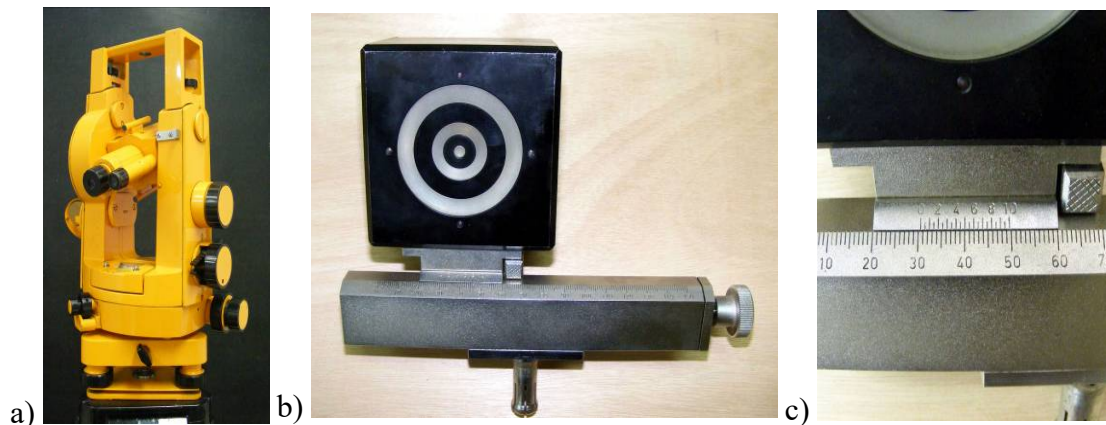
Figure 2. a) theodolite Theo 010, b) and c) a slidable target with a scale and a nonius
