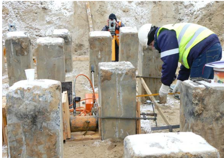
Figure 3. The surveying station for testing lateral load capacity of precast concrete piles
