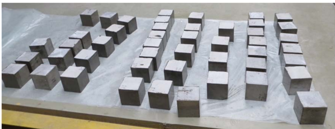
Figure 7. Concrete cubes prepared for testing water-tightness
