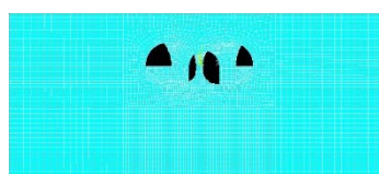
ii). Excavation of right and left pilot heading (up-step)
