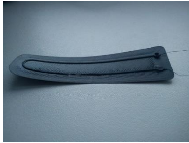
Figure 2. Sample actuator made by 3D printing before activation.
