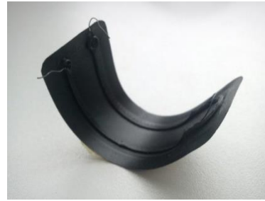
Figure 3. Sample actuator made by 3D printing after activation.
