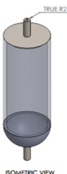
Figure 2. The bubble column reactor
