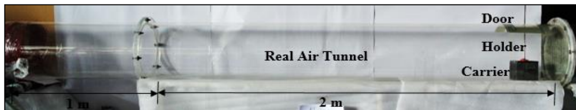
Figure 5. a. The real air tunnel and the position of the carrier.
