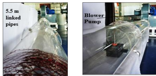
Figure 5.b. The source of the air (blower pump) and the linked pipes (air tunnel).
