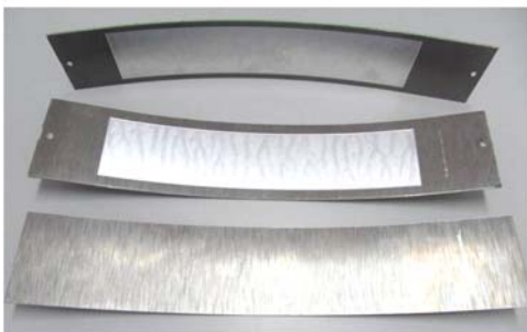
Figure 4. Roll bended-chemical milled workpieces
