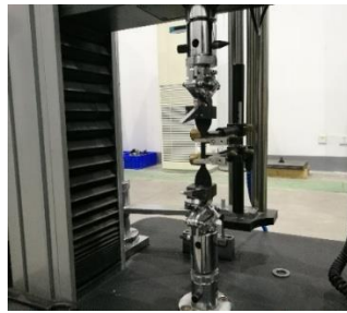
Figure 1. rubber specimen of uniaxial tensile
