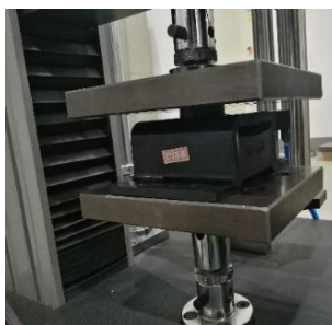
Figure 7. Static test diagram of rubber absorber
