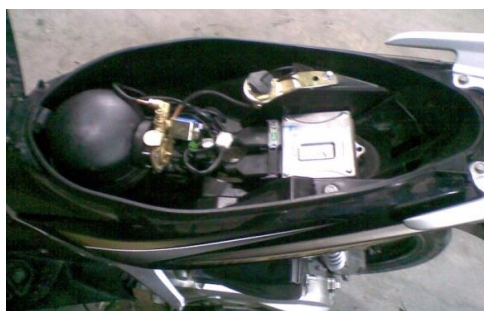
Figure 4. 3-litre LPG storage tank and ECU kit
