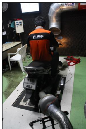
Figure 2. Performance Test on Dynamometer
