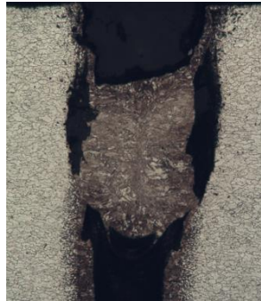
Figure 2. Photo of incision a weld by continuous LR without stabilization LTC settings with burning metal.
