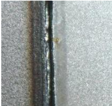
Figure 1. Photo of weld by continuously LR without stabilization LTC settings.
